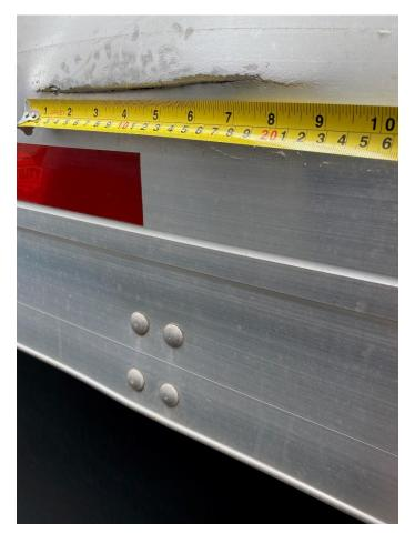
**Note:** The area is greater than 6" and the bend is greater than ¾". The TBR will need replaced per OEM standards.
